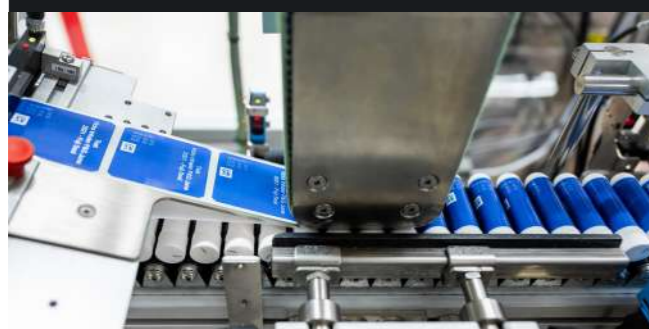
On a prism roller conveyor , products can be transported horizontally, aligned, and labeled.
