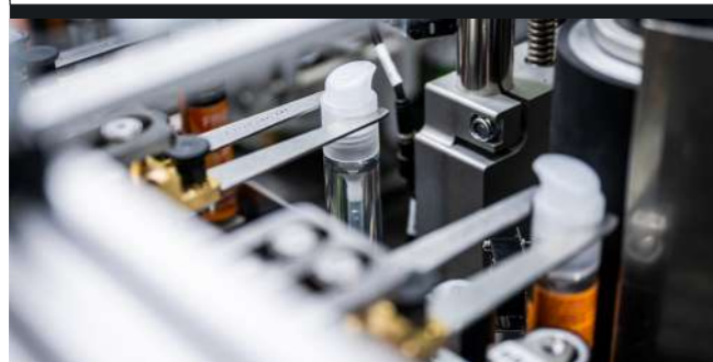
The orbiter aligns the product precisely by gripping it securely and guiding it forward in a controlled manner.
