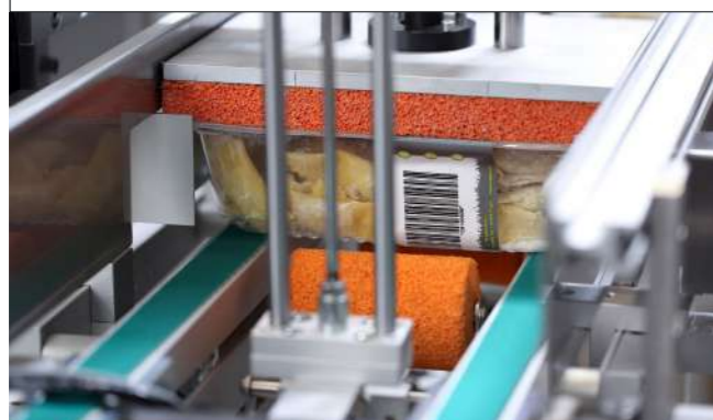
Special pressure rollers ensure secure label adhesion while protecting the product contents.
