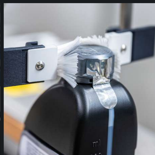
Seal labeling on the canister lid – for tamper-proof product closures.
