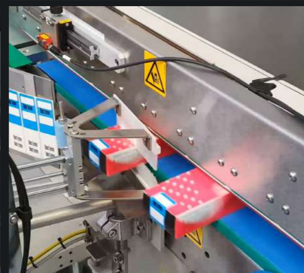
3-sided sealing labeling for products transported in a clamped position.
