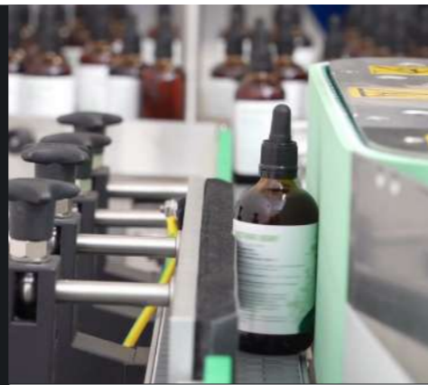
Adjustable side guides stabilize the products during the labeling process.
