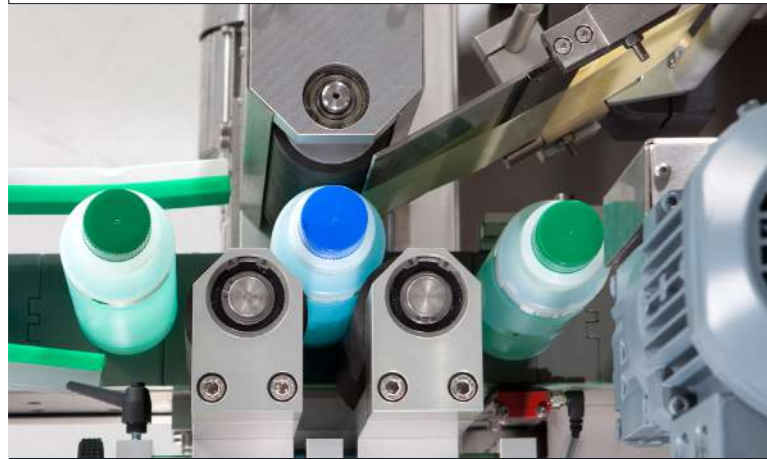
The 3-roller system separates the products and positions the label precisely at a defined reference point.
